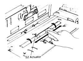
6. Exposure Glass Wipe the exposure glass with the cleaning pen.
